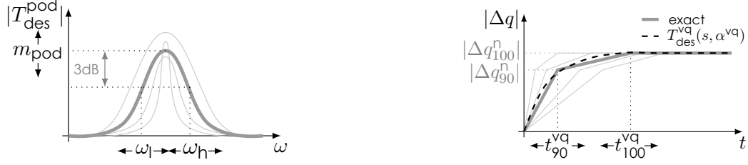
(a) Magnitude Bode plot of bandpass resonator transfer function [20] for active power oscillation damping: \omega_r = \sqrt{\omega_l \omega_h} is the resonance frequency, \Delta\omega_{BW} = \omega_h - \omega_l the filter bandwidth, and m_{pod} the magnitude.
